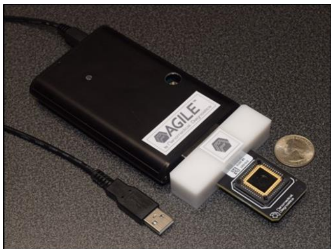
Figure 3: A complete prototype Agile R100 measurement system, including reader hardware (black box), cartridge, and chip, which is USB-compatible in a small form factor.
