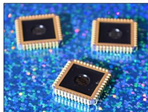
Figure 2: Chip packaging consists of die attach into a 44 pin CQFJ package, followed by Au ball wire bonding and lastly dam and encapsulation using a heat cured epoxy. Several completed Agile chips are depicted with the open cavity available for liquid biological sample insertion.
